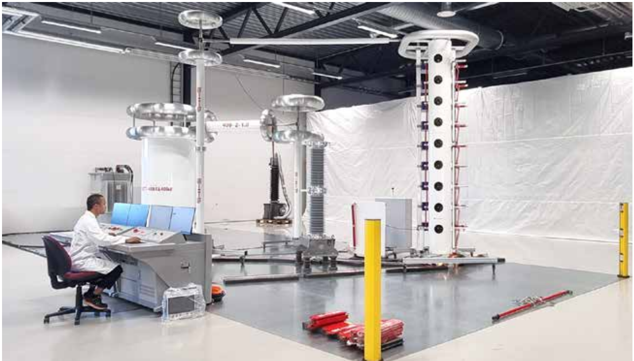
Inhouse high voltage test laboratory, 400kV power frequency and PD test, 900kV 60kJ impulse test system
