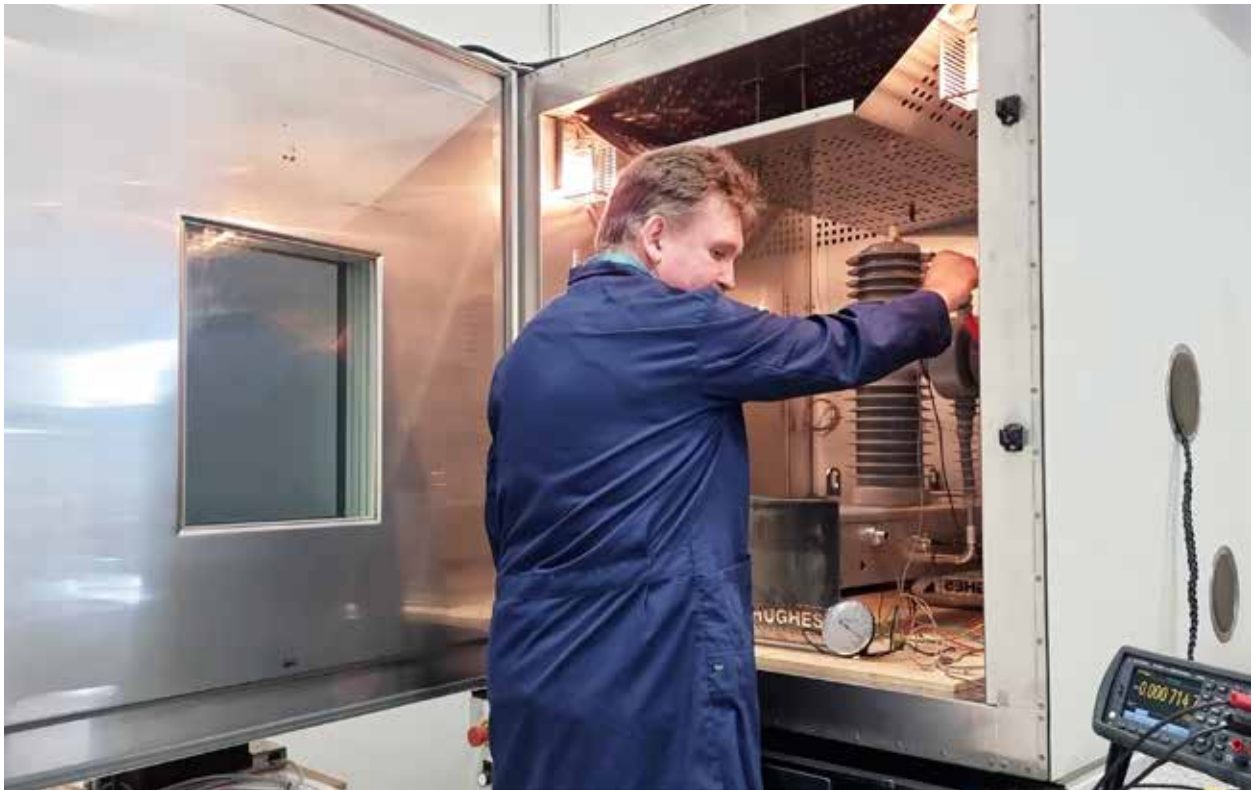
Temperature testing of a switch in the climate chamber, - 80°C to + 180°C
